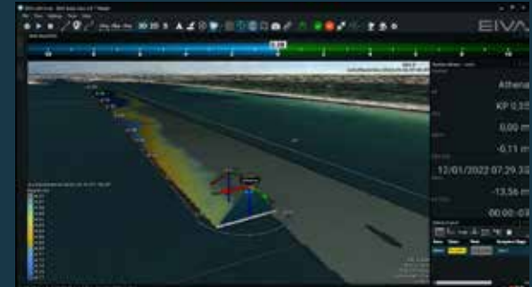
Real-time automatic adaptive runline generation based on the previous surveyed line
