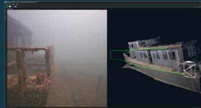
Voyis VSLAM powered by EIVA NaviSuite – Real-time data quality control during ROV visual inspections with Voyis' Discovery camera – Generate high-quality 3D point clouds and navigation trajectory plots for augmented piloting
